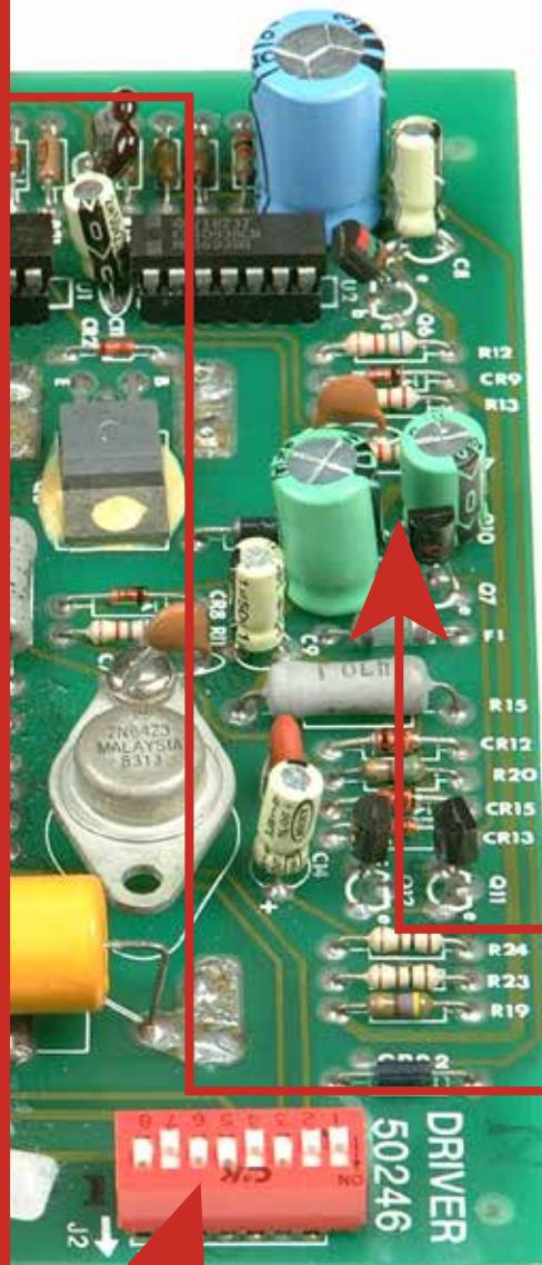
We replace and upgrade all defective low-temperature, low-quality electrolytic capacitors to 105°C. Upgrading from 85°C to 105°C more than doubles the life of your capacitors.
